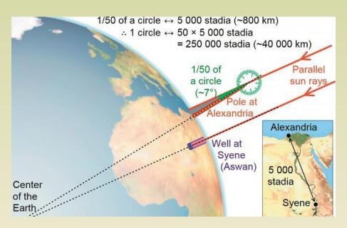
On the day of Summer solstice Eratosthenes measured the angle of a shadow cast by a stick at noon in Alexandria. Sunlight fell at an angle of about 7.2°. In Syene the Sun was directly overhead.
